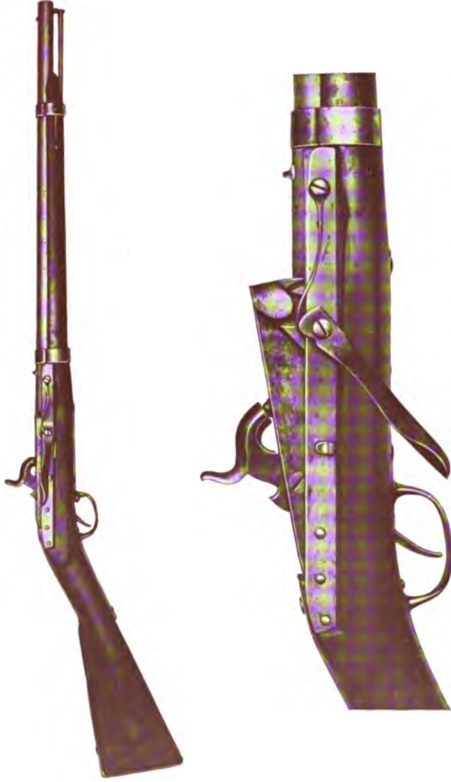
Hall Carbine. 1843 to 1852. Known as "North's Improvement." Length 40 inches. Length of barrel 21 inches. Caliber, 54. North's improved method of operating the receiver.
